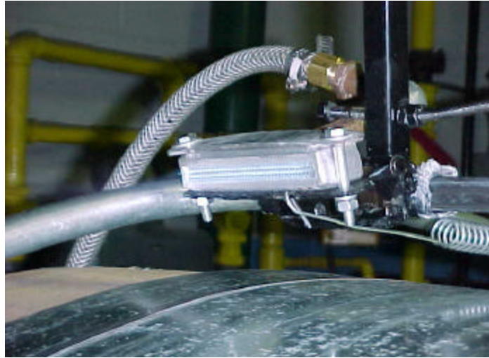
Figure 10. Flame treatment burner
